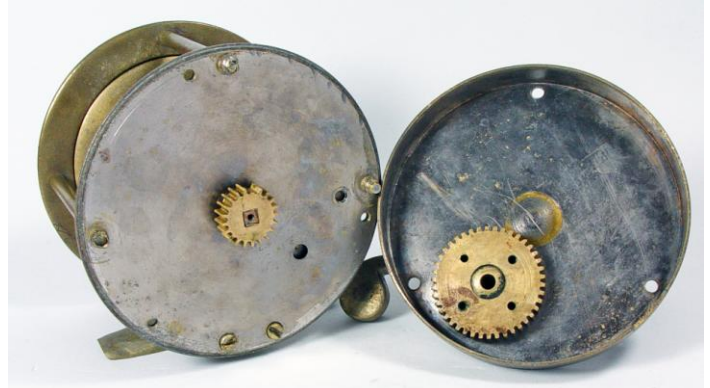
The inside of the brass reel. A missing brake spring was attached at the hole near the pillar and its pin extended through the hole near the pinion. The brake lever rim groove is near the main gear but is barely discernible in the photo.
