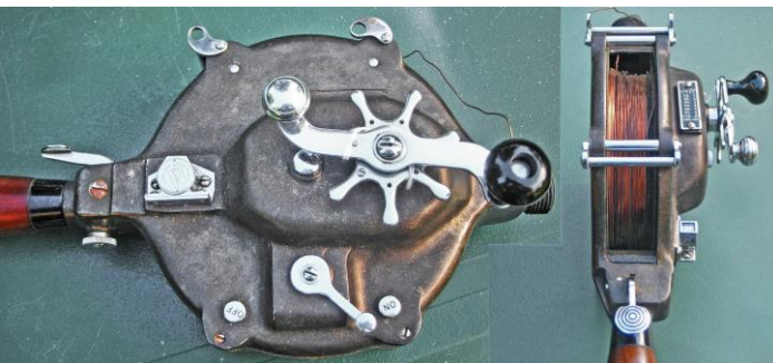
Two views of a multiplying combo bearing a Veeder line counter. The raised-pillar reel has a star drag. (Photos courtesy of James O’Brien)
