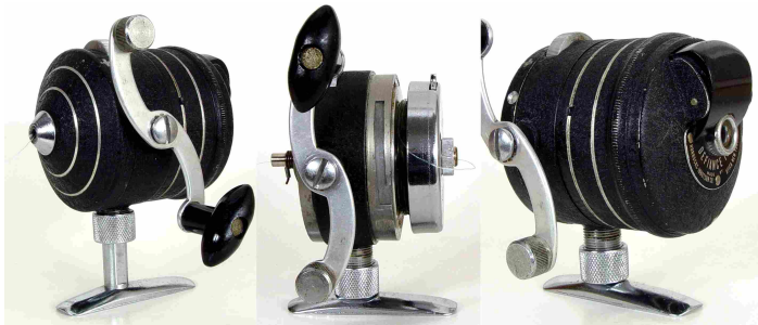
Figure 11. The dual-function H-I "Defiance" reel. (Left) Ready for mounting under a spinning rod, with the line exiting from the spool through a central tube. (Center) The reel with both caps removed. The spool and line pickup, based on Small's inventions, are similar to those in the earlier H-I models. (Right) The other end of the reel. The line can be fed from this end for spin-casting from a casting rod. The large button brakes the spool. The foot is visible in extended (left) and retracted positions.
