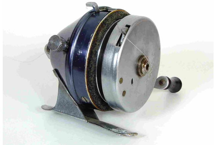
Figure 9. The Aristocast with its rear cover removed to show the Cormorant-like mechanism inside. The line enters the hollow central shaft at the front of the reel, exits the shaft at the rear, and turns forward to be wound onto the spool.
