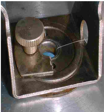
Figure 3. The center of the reel, viewed from below. The line exits through a hole in the foot bracket. A thumbscrew adjusts drag against the reel cup.
