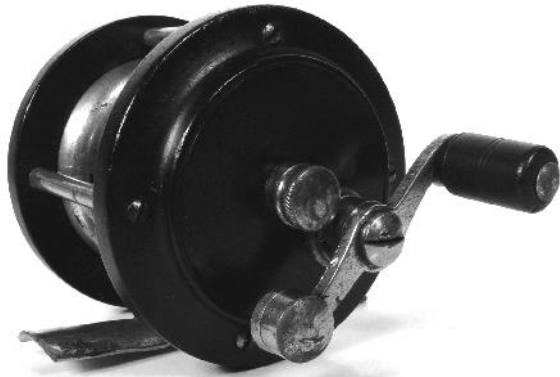
The sideplates of this Kopf-footed reel are made of rubber or celluloid.
