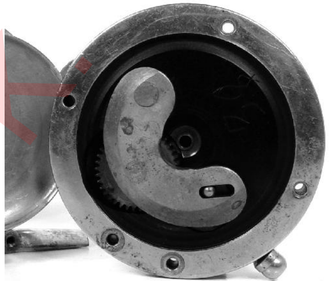
An "adaptation" of Kopf's clutch in a later Julius vom Hofe casting reel.
