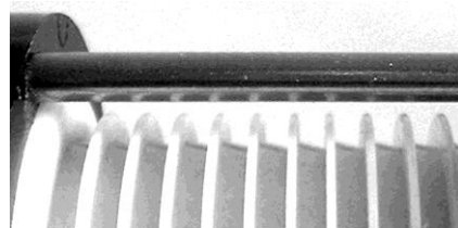
Closeup of the “Keahoni” spool grooves, showing the slanted bottoms.
