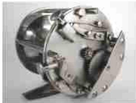
The American Reel Co. reel with the headcap removed to show the click and drag. The 10X multiplying ratio is produced by a conventional train of four spur gears.
